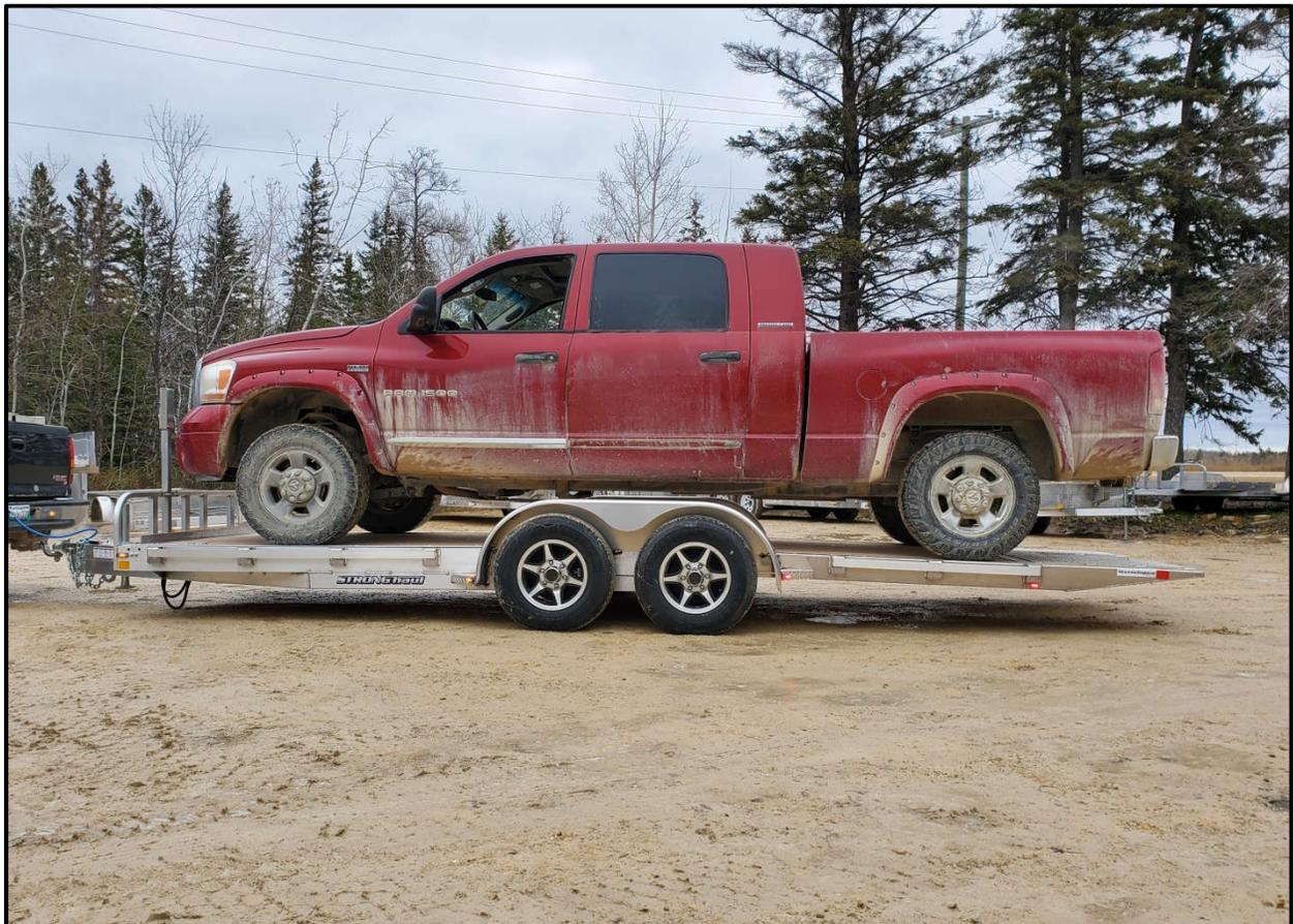
All trailers released after this prototype have added gusseting and reinforcements to help prevent the tilt deck from deflecting to this extent, but all tilt deck models will still have some spring back and it is important to take this into account when unloading.
